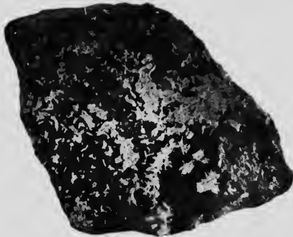
Polished surface of ore from Sunnyside mine, No. 3. White areas are arsenopyrite well crystallized. Grey areas pyrrhotite, without crystallographic outline. Dark areas ground mass of diopside and quartz.
